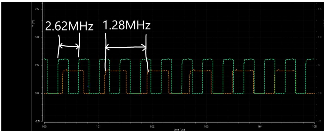
VDD transient analysis (Out @ 2, 3V) at 27°C with a load of 5Ω
