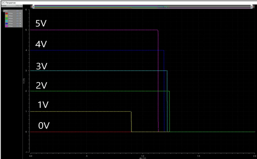
VDD parametric DC analysis of the cascade comparator output
